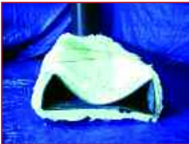
12"x36" rectangular, 16 Ga., welded, carbon steel duct with generic "wrap" insulation – after 2000°F (simulated grease fire) for 30 minutes.
