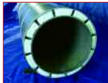
24" ZeroClear™ after 2000°F (simulated grease fire) for 30 minutes.
